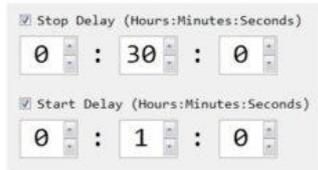
In this example, the output relay comparator turns on after one minute (T1) and turns off after 30 minutes (T2). You can put the timers to zero when Be48 is used in particular applications. The range of the timers spans from one second up to 24 hours. This picture makes it clear.
